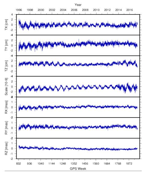
Figure 2: Transformation parameters between the input daily combined EPN SINEXs and the EPN multi-year SINEX output of the combination. These 7 parameters shows the reference frame alignment of the daily combined EPN SINEXs with respect to the EPN multi-year solution
