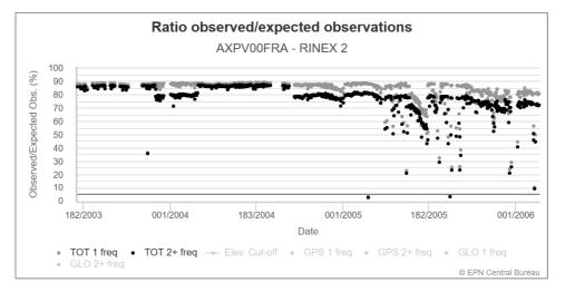
Figure 4: Time series of the ratio observed versus expected RINEX observations between summer 2003 and 2006 at AXPV00FRA.
