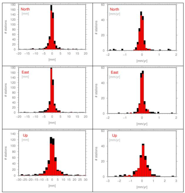
Figure 6: Histogram of the position (left) and velocity (right) differences between the EPN solution C1950 and the IGS solution IGS17P21
